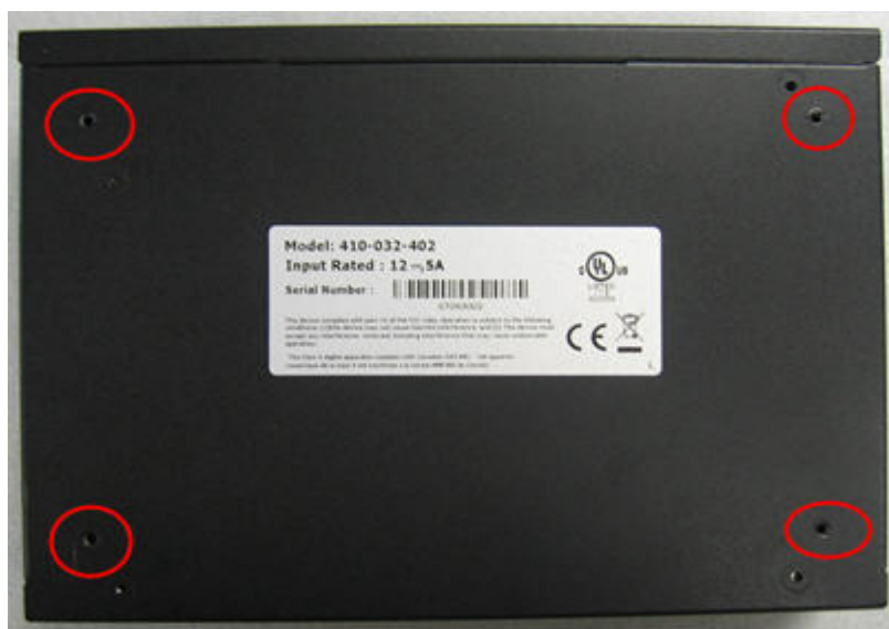
Figure 19 Screw holes for rubber feet installation on bottom of unit
